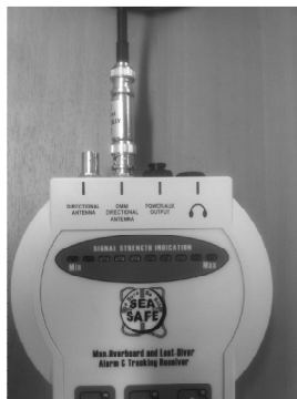
Receiver with attenuator and Tracking antenna plugged into Omni-Directional Antenna Port
