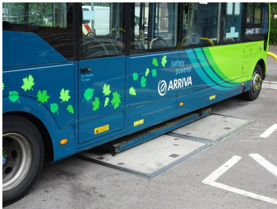
Figure 1: Bay No1 with the induction loop plate lowered over the induction pad.
