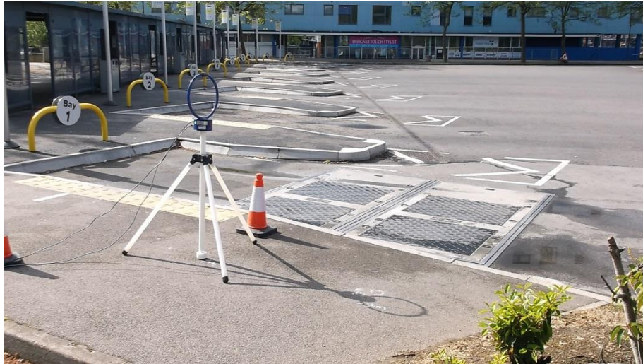
Figure 2: Unoccupied Bay No1 with the 4 induction pads visible. (Loop antenna 3 m from centre of pads – initial measurement for interim report)
