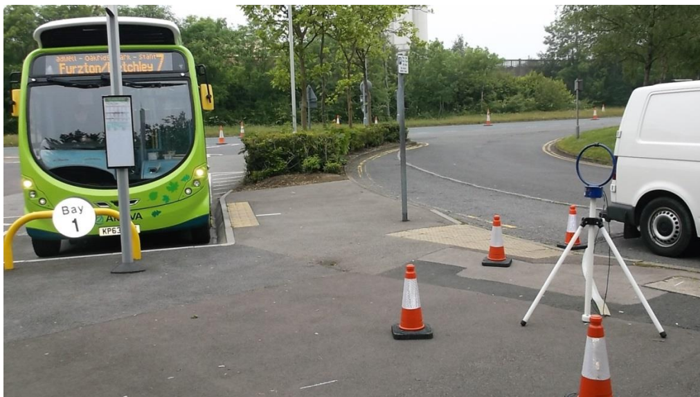
Figure 6: Initial 10m antenna location segregated from passenger movements.
