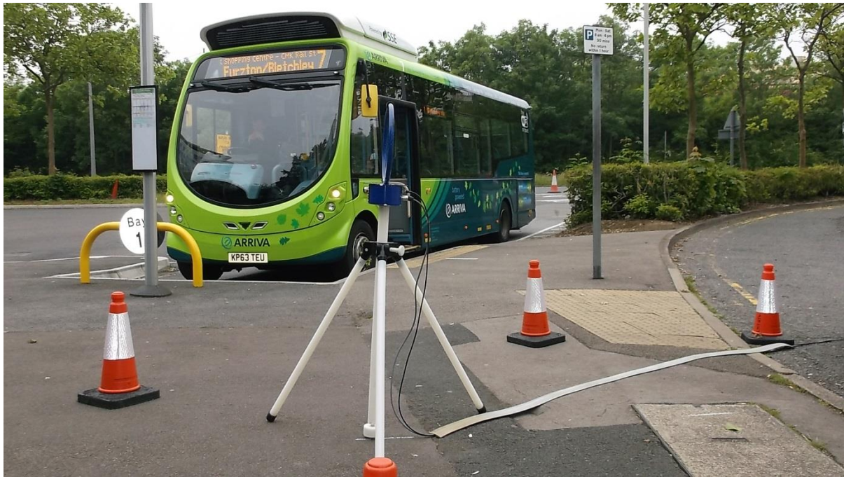
Figure 3: Loop orientation for maximum received signal from the induction pads.
