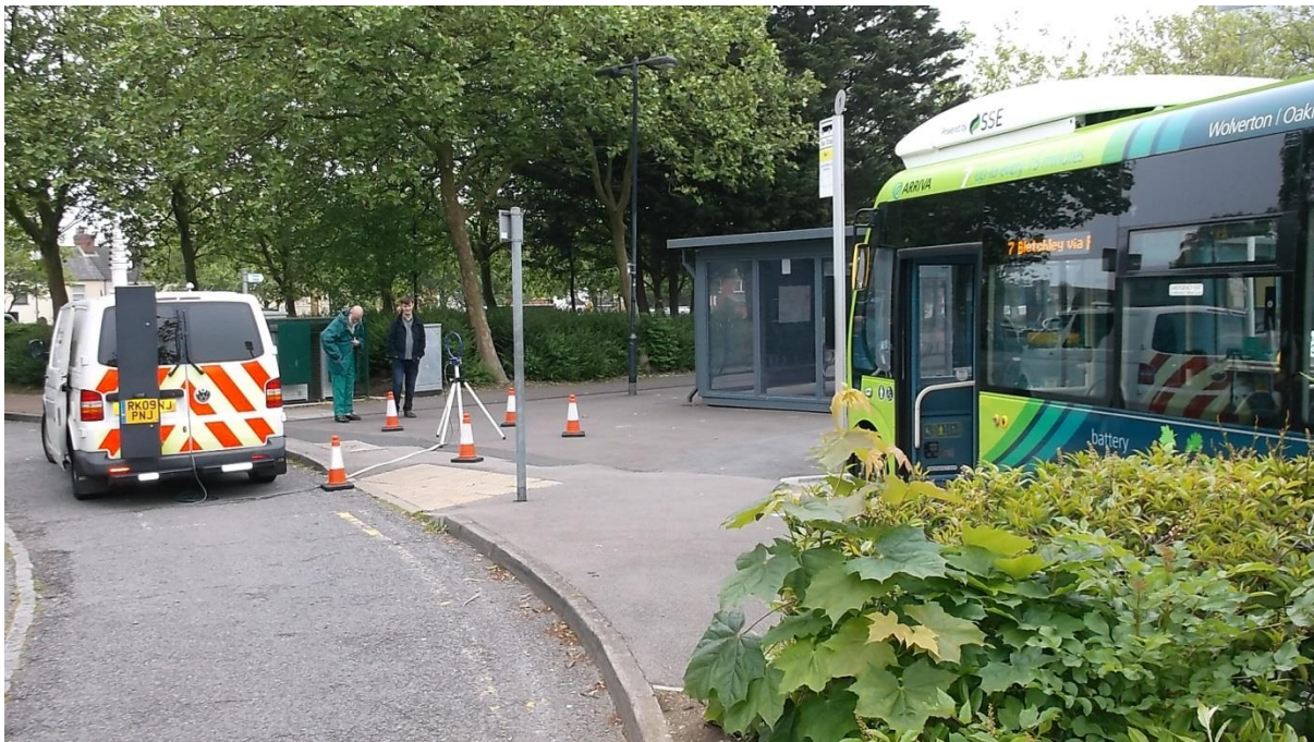
Figure 8: Antenna in location 1 measuring emissions during the bus charging cycle.
