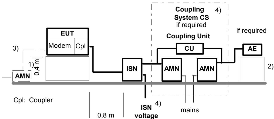
333 NOTE 1 Distance from EUT to the reference ground plane (vertical or horizontal).
