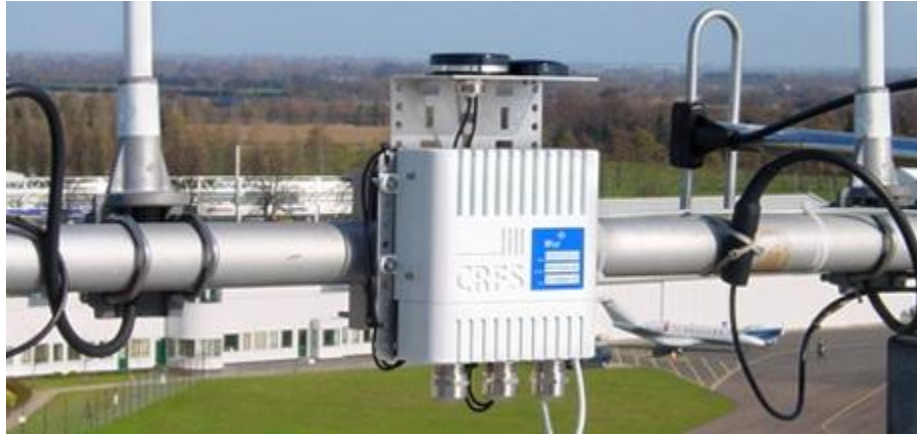
Figure 4 – A mounted RFeye measurement device. Antennas can be seen to the left and right.
